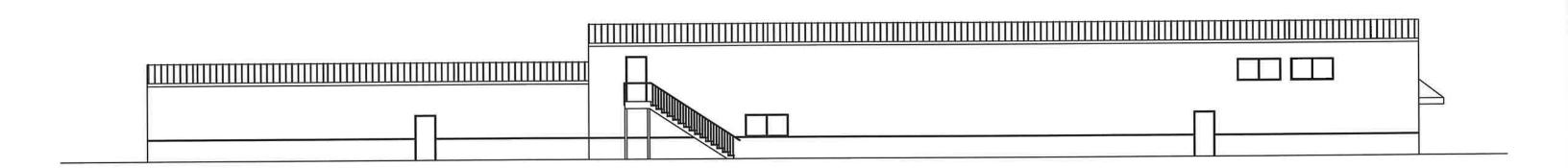
1/2" / 12 slope roof all draining to the back of the building so nothing over garage doors
